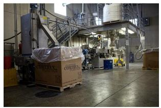
Manufacturing lines include both reactive twin-screws and single-screw technologies.
